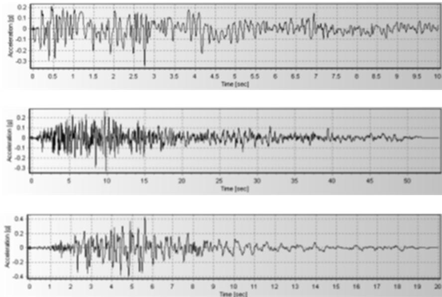
Fig. 4. Time history of ground motions in stream: top–Rudbar, middle–Bam and bottom–Tabas
