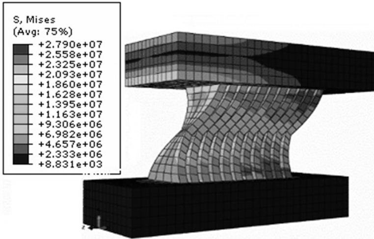
Fig. 6. Stress in ADAS damper in model M15-6
