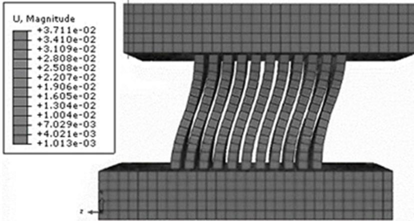
Fig. 5. Displacement in ADAS damper in model M15-6
