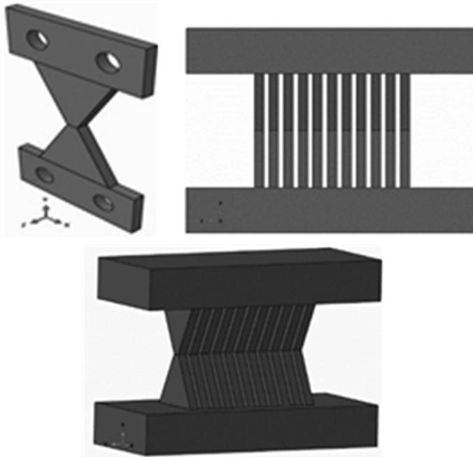
Fig. 3. Abaqus model of ADAS damper
