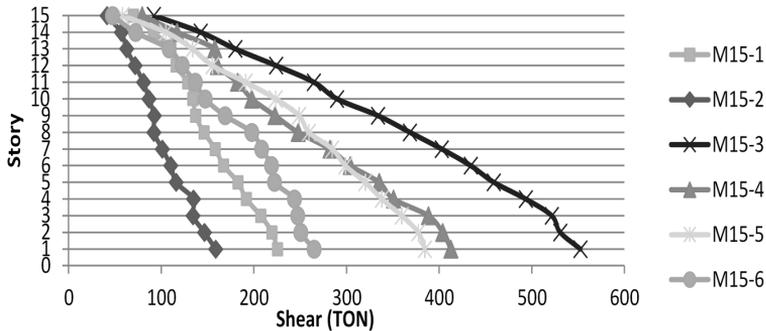
Fig.7. Story Base Shear for 15-story structure
