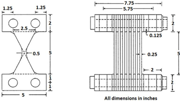
Fig. 1. Arrangement of ADAS devices
