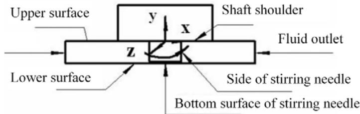
Fig. 2. Schematic of computational zone
