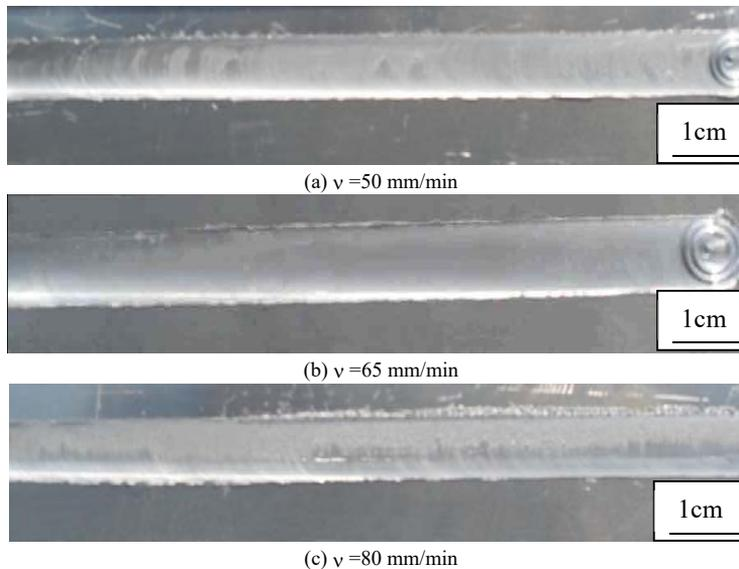
Fig. 1. Effect of different welding speed on joint quality
